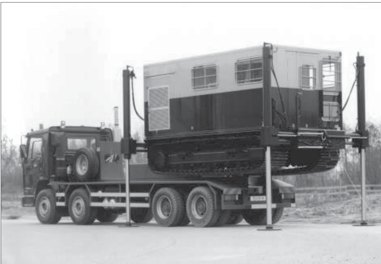
Fig. 20 Cone Penetration Testing Unit, The Netherlands
